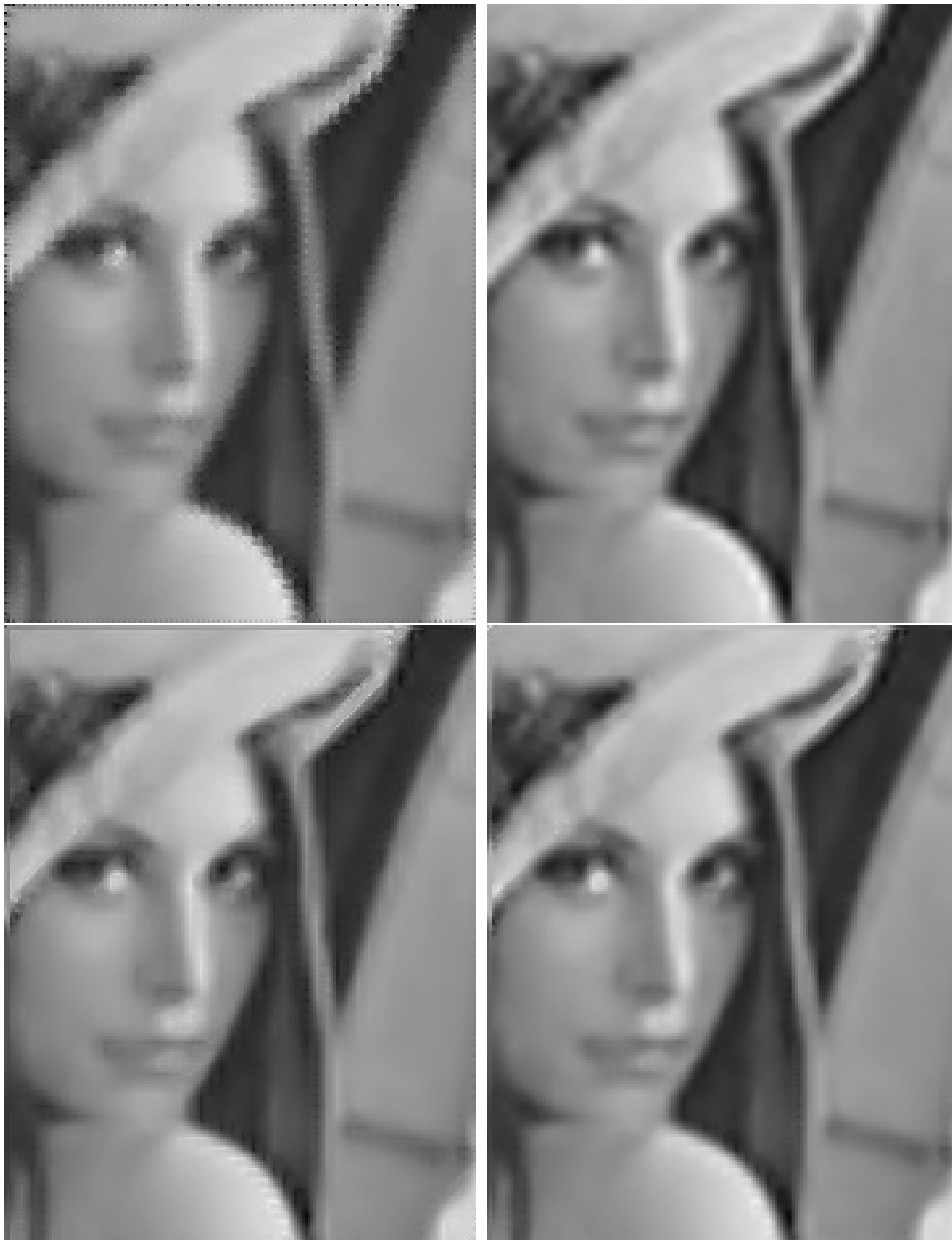
Figure 7. Resulting images for image interpolation. Interpolation to four times as many pixels. Top left: result from the method of Bertalmio et al. [4]. Top right: result from bicubic interpolation. Bottom left: result from minimization using the Euler equations. Bottom right: result from minimization using the H^1 gradient.
