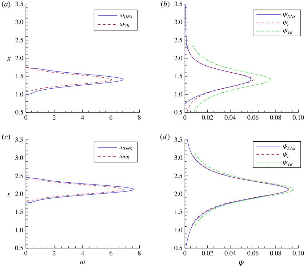
FIGURE 14. (Colour online) The same as in figure 13, but for the profiles along the  $x$ -axis through the centre of the vortex (at  $r = R_0$ ).  $D_w/D = 1.75$  (a,b) and  $D_w/D = 3$  (c,d).
