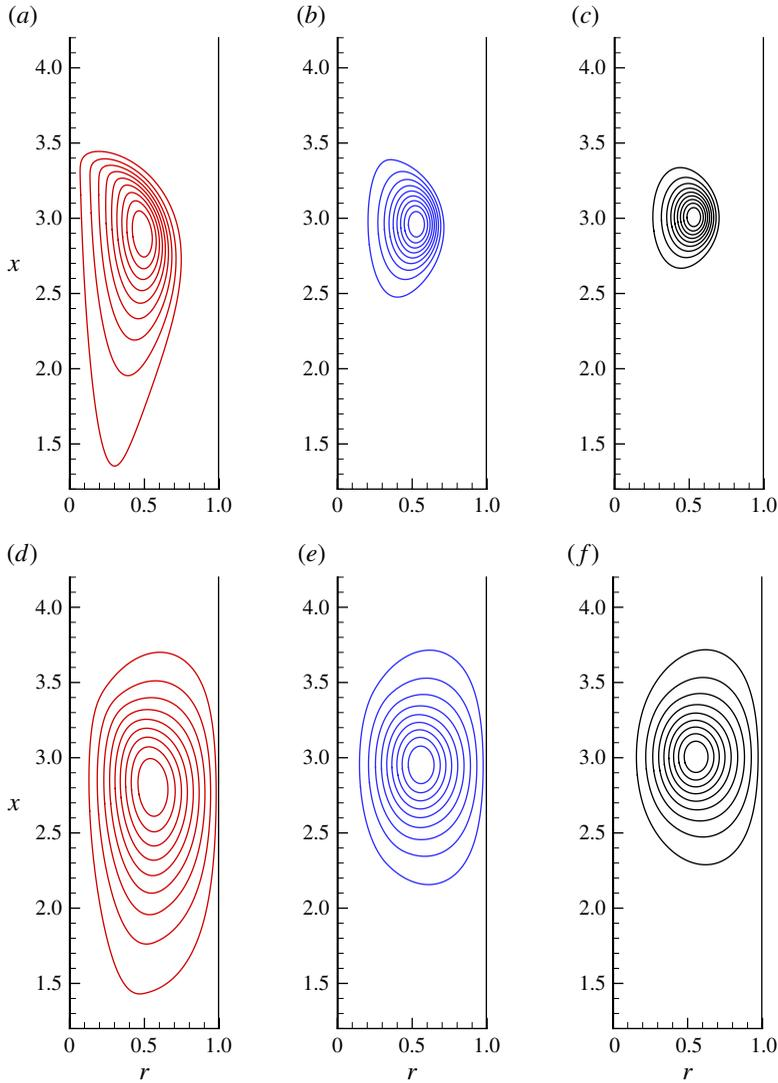
FIGURE 10. (Colour online) Contours of (a–c) normalised vorticity  $\omega/\omega_{max}$  and (d–f) the corresponding normalised streamfunction  $\psi/\psi_{max}$ , for the time instant  $\tau = 15$  and confinement parameter  $D_w/D = 2$ ; (a,d)  $Re_D = 500$ , (b,e)  $Re_D = 1700$ , (c,f)  $Re_D = 3400$ . The values of  $\omega/\omega_{max}$  and  $\psi/\psi_{max}$  are shown from 0.1 to 0.9 with increments of 0.1.
