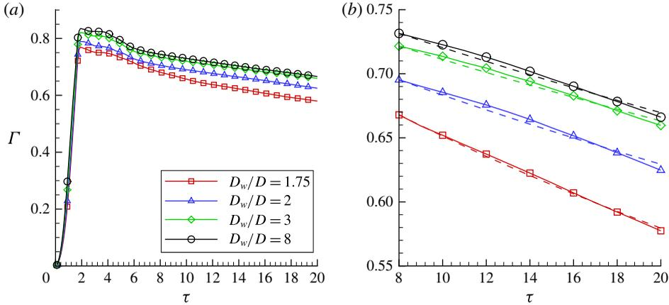
FIGURE 9. (Colour online) (a) Time evolution of the vortex ring circulation for four values of the confinement parameter  $D_w/D$ . (b) Close-up corresponding to the post-formation phase of the vortex ring evolution. Dashed curves show the results inferred from (3.11) suggested by Stewart *et al.* (2012).  $Re_D = 1700$ .
