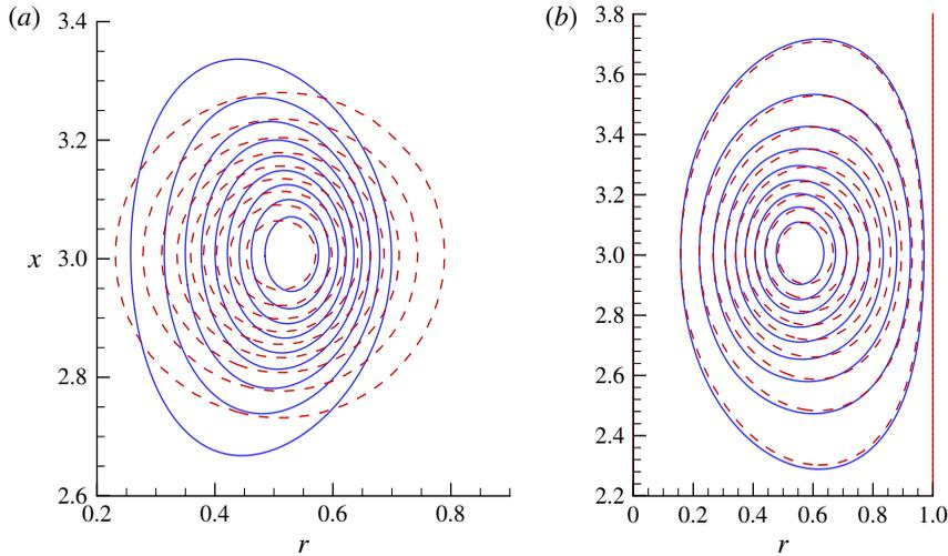
FIGURE 18. (Colour online) Contours of normalised vorticity  $\omega/\omega_{max}$  (a) and corresponding normalised streamfunction  $\psi/\psi_{max}$  (b), obtained by DNS (blue solid curves) and the vortex ring model (red dashed curves). The values of  $\omega/\omega_{max}$  and  $\psi/\psi_{max}$  are shown from 0.1 to 0.9 with increments of 0.1.  $Re_D = 3400$ ,  $D_w/D = 2$ ,  $\tau = 15$ .
