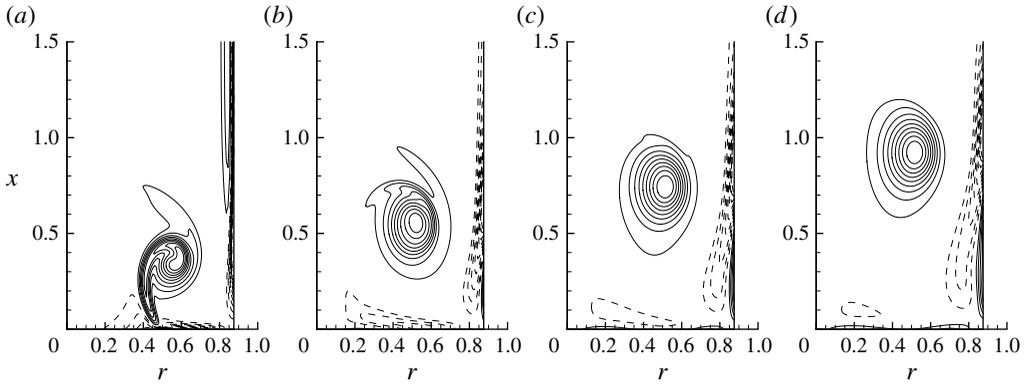
FIGURE 5. Contours of vorticity  $\omega$  at the early stage of formation of the vortex ring in a tube. Dashed curves show contours of negative vorticity. Times: (a)  $\tau = 2$ , (b)  $\tau = 3$ , (c)  $\tau = 4$ , (d)  $\tau = 5$ ;  $Re_D = 1700$ ,  $D_w/D = 1.75$ .
