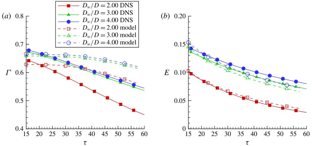
FIGURE 19. (Colour online) Time evolution of the circulation  $\Gamma$  (a) and energy  $E$  (b) of the vortex ring, as inferred from DNS data and predicted by the model for three confinement parameters  $D_w/D$ .  $Re_D = 3400$ .
