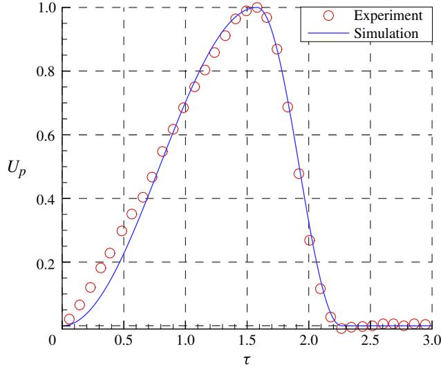
FIGURE 4. (Colour online) Piston velocity  $U_p(\tau)$  used for numerical simulations (solid curve) and experimentally observed piston velocity reported by Stewart *et al.* (2012) (symbols).
