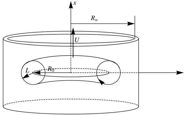
FIGURE 1. Schematic of a vortex ring in a tube.
