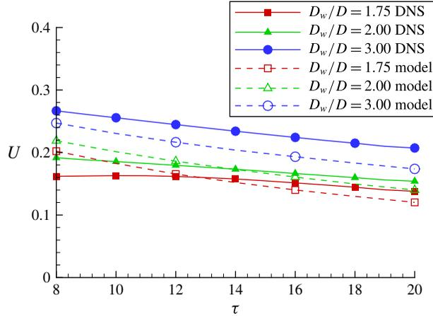
FIGURE 17. (Colour online) Time evolution of the translational velocity  $U$  of the vortex ring. Comparison between DNS data and the model predictions (4.5) for three confinement parameters  $D_w/D$ .  $Re_D = 1700$ .
