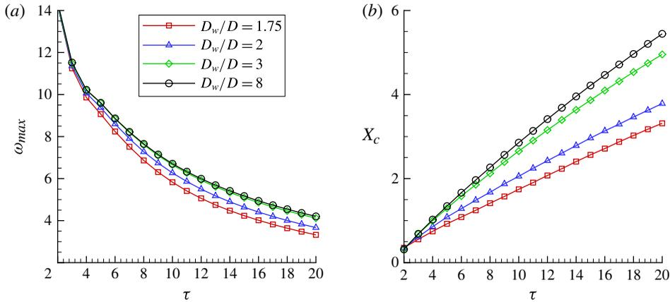
FIGURE 7. (Colour online) Time evolution of maximum vorticity  $\omega_{max}$  and streamwise position of the vorticity centre  $X_c$  corresponding to the maximum vorticity;  $Re_D = 1700$ .
