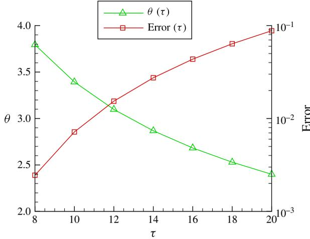
FIGURE 15. (Colour online) Time evolution of parameter  $\theta$  assumed in the model (see (2.24)) and corresponding maximum relative error intrinsic to the model (see (2.30)).  $Re_D = 1700$ .
