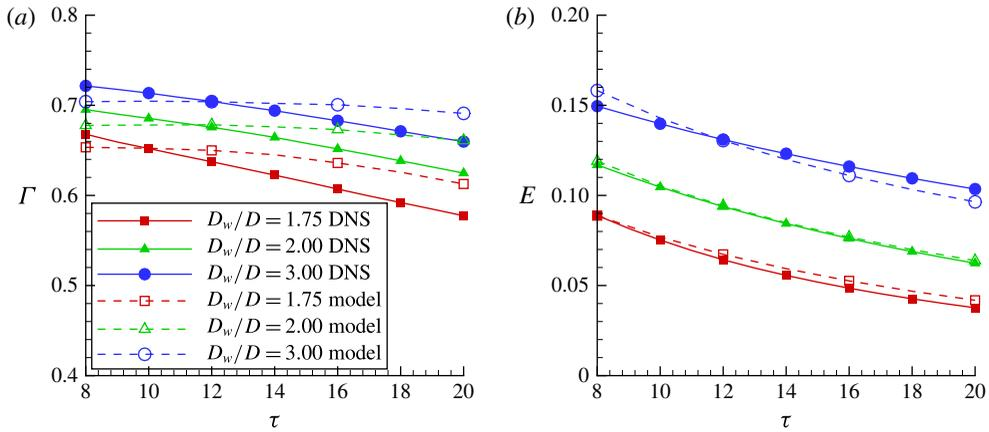
FIGURE 16. (Colour online) Time evolution of the circulation  $\Gamma$  (a) and energy  $E$  (b) of the vortex ring obtained by DNS and the model for three confinement parameters  $D_w/D$ .  $Re_D = 1700$ .
