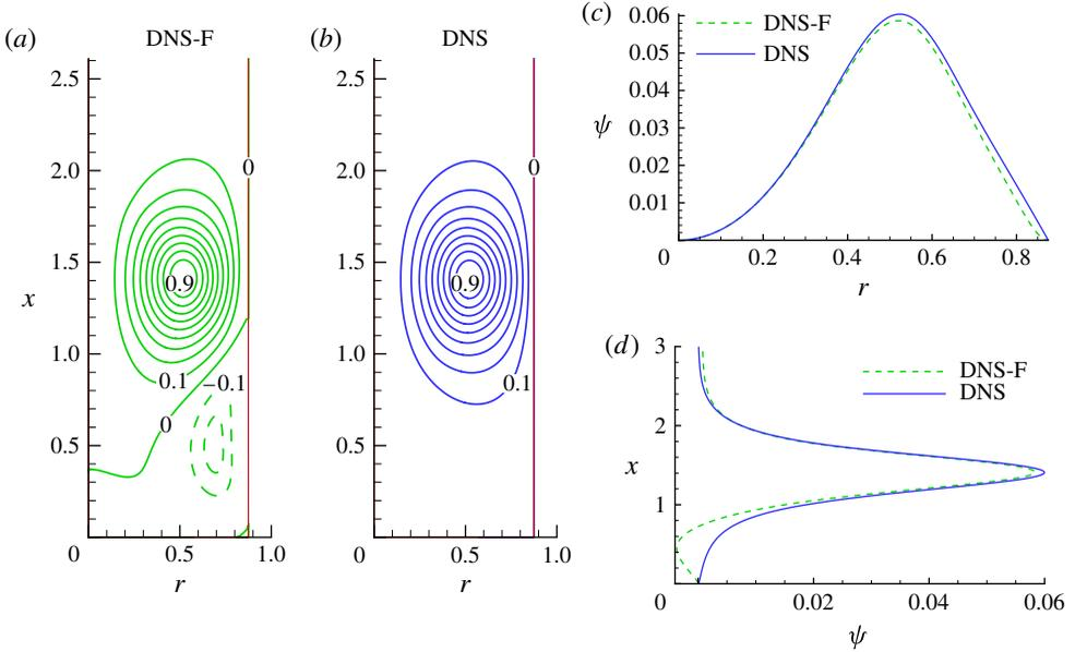
FIGURE 11. (Colour online) Contours of normalised streamfunction  $\psi/\psi_{max}$  obtained by solving (2.2) numerically with the right-hand side term corresponding to the full DNS vorticity field (a, DNS-F) and to the vorticity inside the vortex ring core ( $\omega/\omega_{max} \geq 0.05$ ) (b, DNS). Streamfunction profiles through the centre of the vortex: (c) along the  $r$ -axis ( $x = X_c$ ), (d) along the  $x$ -axis ( $r = R_0$ ).  $Re_D = 1700$ ,  $D_w/D = 1.75$ ,  $\tau = 8$ .
