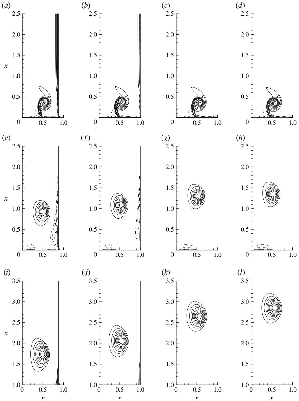
FIGURE 6. Contours of the normalised vorticity  $\omega/\omega_{max}$  at various time instants and confinement parameters. Times: (a–d)  $\tau = 2$ , (e–h)  $\tau = 5$ , (i–l)  $\tau = 10$ . Parameters: (a,e,i)  $D_w/D = 1.75$ , (b,f,j)  $D_w/D = 2$ , (c,g,k)  $D_w/D = 3$ , (d,h,l)  $D_w/D = 8$ ;  $Re_D = 1700$ . The values of vorticity increase from  $-0.3$  to  $0.9$  with increments of  $0.1$ ; dashed curves show contours of negative vorticity.
